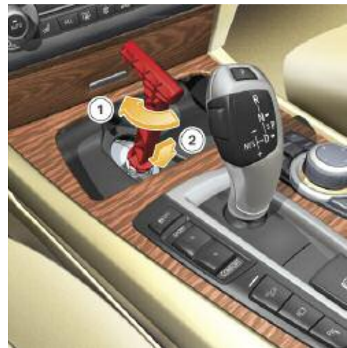
Releasing parking lock on F01/F02
